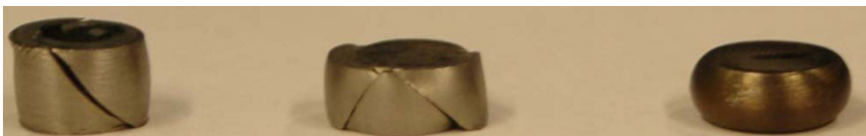
图4 钛合金不同镦粗试样 Fig.4 Titanium alloy specimens produced by different upsetting processes
